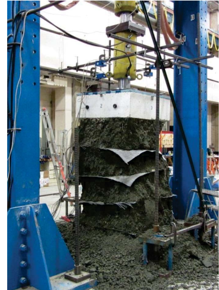
TF-10 at failure with S_v = 15\frac{1}{4} inches, T_f = 4,800 lb/ft, and VDOT 21A material. (Nicks et al., 2013)
