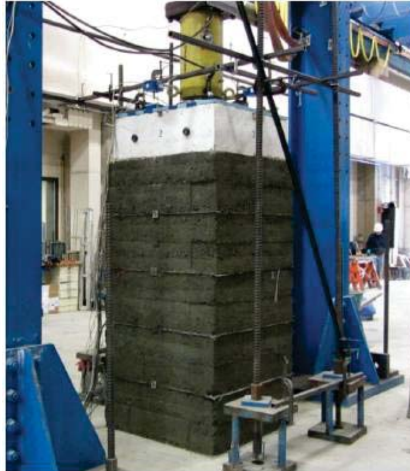
Unfaced GRS Mini-Pier (Nicks et. al, 2013)
