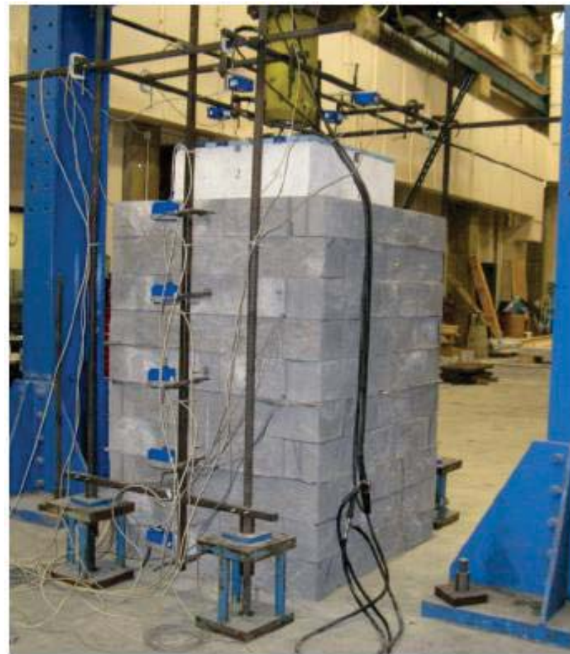
Faced GRS Mini-Pier (Nicks et. al, 2013)
